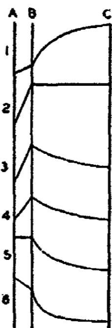
FIG. 2. SCHEMATIC REPRESENTATION OF THE COURSE OF THE POTENTIAL CURVES IN VARYING CONCENTRATIONS OF ThCl 4
